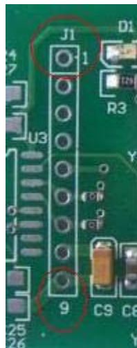
Figure 1 – YHY502CG J1 PinOut TOPView
