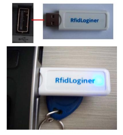
When plug the YHY202D reader to the PC's USB port, the system will recognize it as HID keyboard device.
